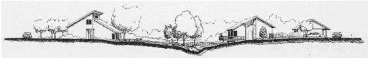
Cross-sectional sketch of village homes housing, bioswales and front yards with walking paths between.
